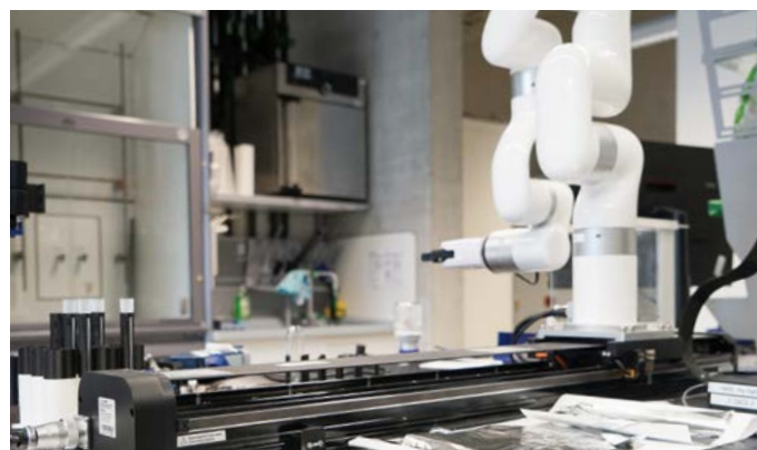
Automated for better batteries: In Prof. Helge Stein's laboratories, robots mix various active powders and liquids to create battery pastes, so-called slurries. These are then applied to a copper foil (above). Combined with further tests, AI-assisted data evaluation and temperature analyses, the system accelerates the development of high-performance battery materials.
